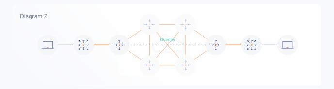
The overlay in this example could support any of the following protocols it doesn't just have to be LISP with VXLAN encapsulation (which are specific to Cisco's implementation of SD-Access);
