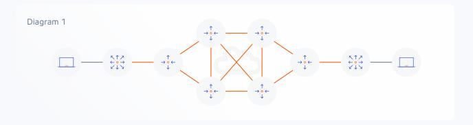
However from a logical standpoint, the following diagram shows the overlay network running on top of the underlay network. As you can see the logical topology has been greatly simplified.
